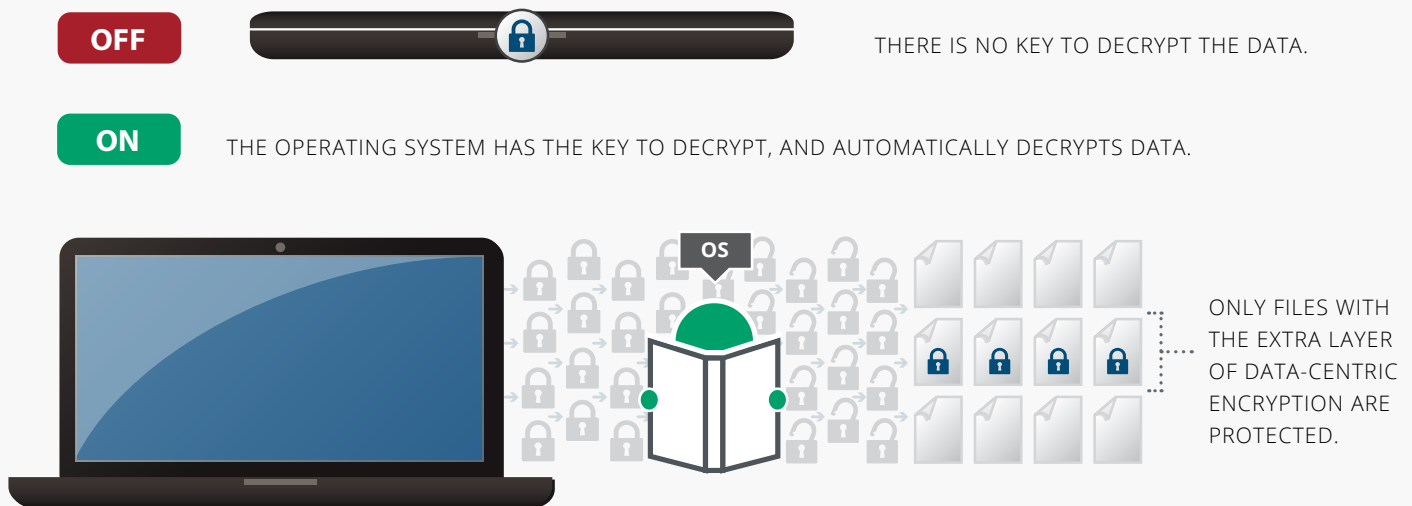
FIGURE 3 —WHOLE DISK ENCRYPTION SECURITY WHEN OPERATING SYSTEM IS POWERED ON VS. OFF.
